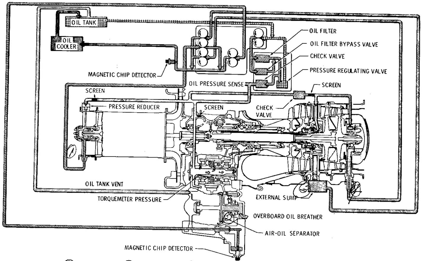
● SUPPLY AND BYPASS OIL    ● PRESSURE OIL    ● SCAVENGE OIL    ● TORQUE MODULATED PRESSURE    ● SCAVENGE RETURN    ● VENT TO ATMOSPHERE
