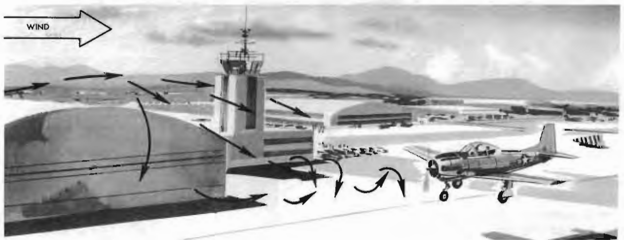
Figure 10-7. Building or other Obstructions on Windward Side of Landing Area May Cause Turbulent Air
