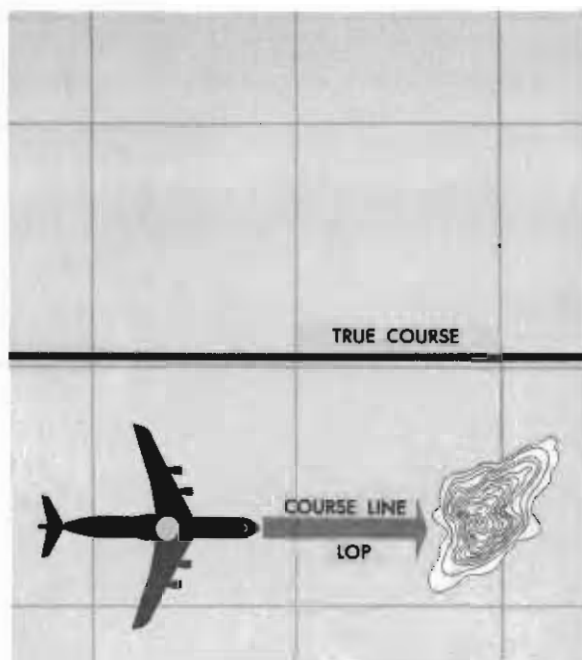
Figure 6-5. LOP Parallel to Track Is Course Line
