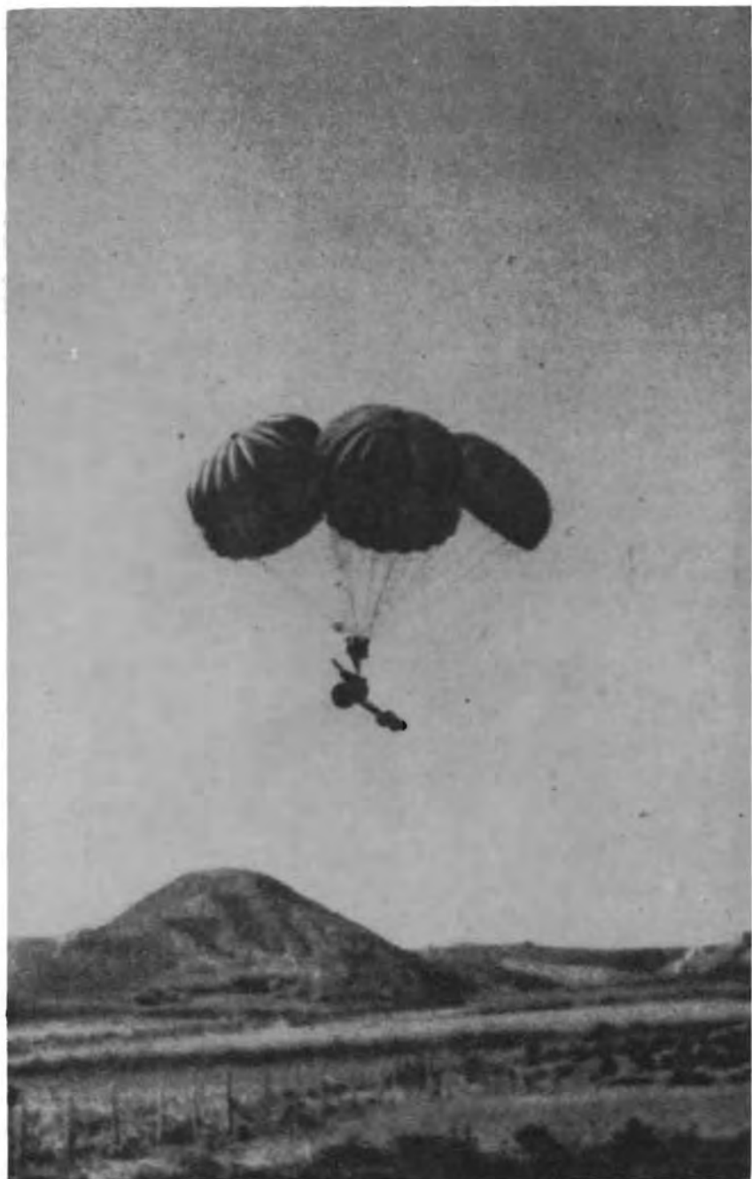
Figure 41. Antitank gun, attached to five parachutes, is dropped over Crete.
