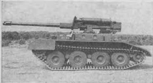
Figure 76. The 90-mm full-tracked, self-propelled gun M56.
