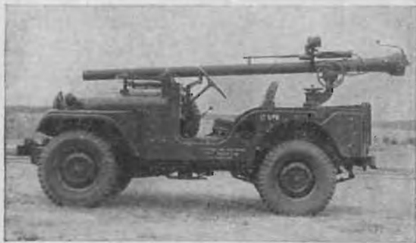
Figure 75. The 106-mm rifle mounted on 1/4-ton truck.
