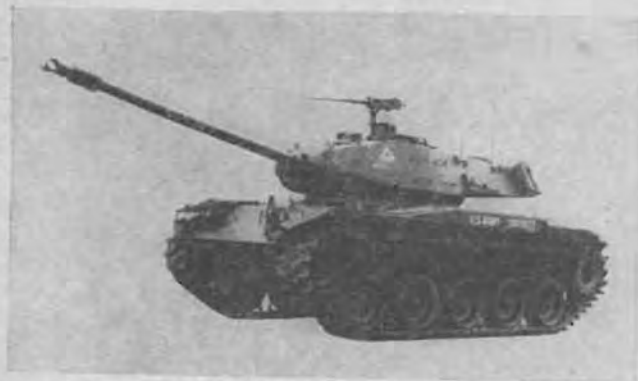
Figure 94. Light tank M41A3. Weight, 26 tons; primary armament 76-mm gun.
