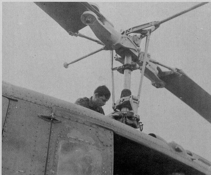
The swash plate is loose
