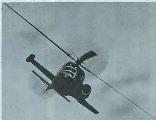
The XH-51A compound (winged) helicopter has set a new world's speed record for rotorcraft. The Lockheed-developed rigid rotor aircraft reached a top speed of 302 miles an hour in tests for the U.S. Army Aviation Materiel Laboratories. The four-blade XH-51A is 32 feet long, 9 feet high, and has a rotor diameter of 35 feet. Wing span is 17 feet. The 5000-pound vehicle is powered by a turbine engine and an auxiliary jet engine (seen on left wing).
