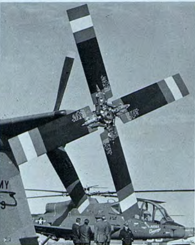
The AH-56A features a 10' tail rotor and pusher prop.
