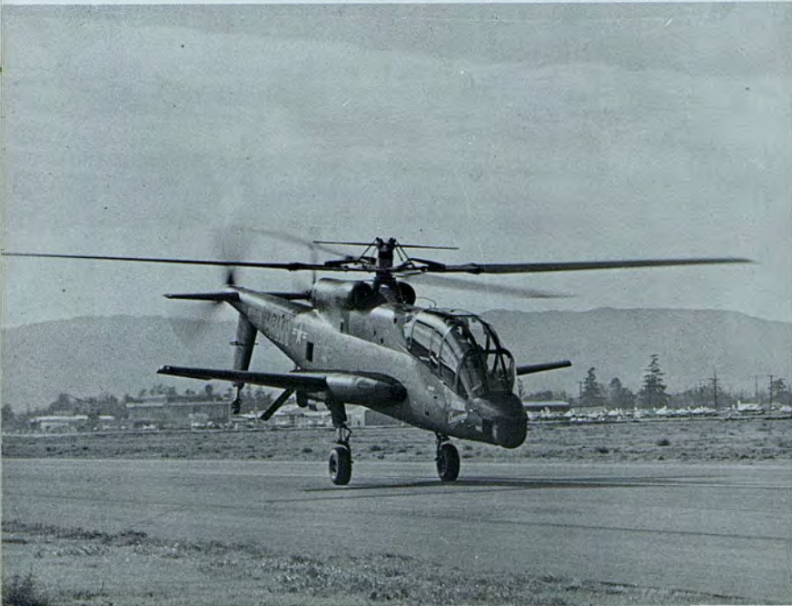
In STOL configuration, craft can carry 7 tons of armament.
