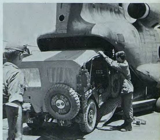
Ushering a jeep into a well balanced "seat" in a Chinook requires expertise from all parties, particularly the flight engineer and the crew chief.
