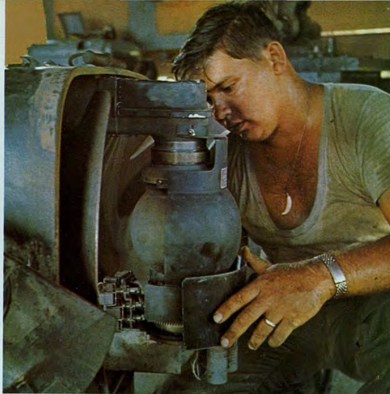
One of the crew members of the searchlight battery checks the Xeon lamp.
