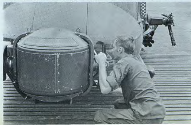
SP4 Jackie Easley pulls maintenance on the FLIR sensor. If this 260-pound piece of equipment fails to function, costly errors result.
