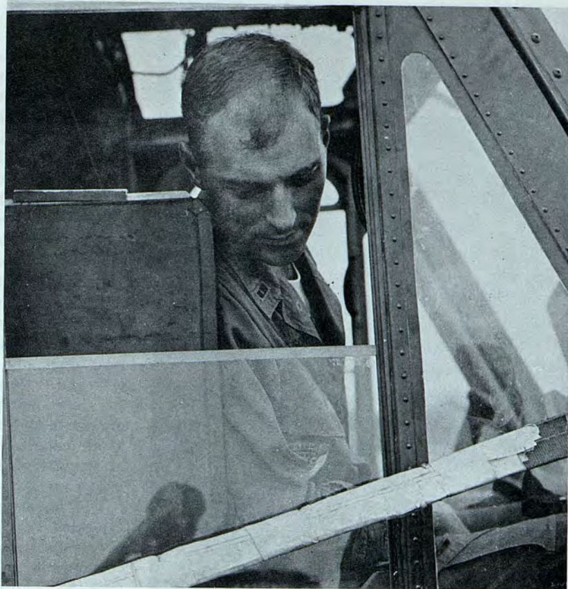
WO Nelson checks cuts made by mechanics while tracking rotor blade alignment.
