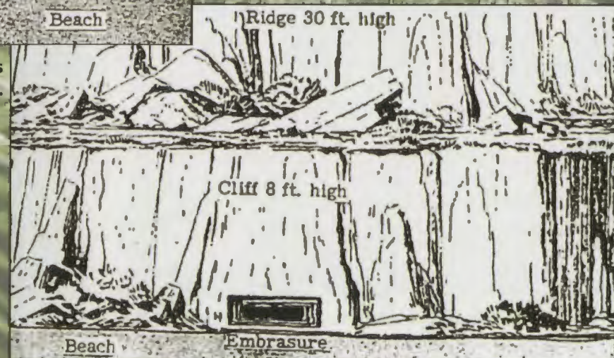
Principles of Construction: Dig as deep as possible and keep as low a profile as possible.
