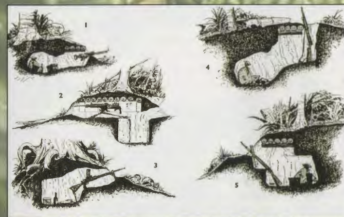
Examples of small Japanese individual fighting positions: (1) 7.7mm Aircraft Machine Gun modified for ground use; (2) 7.7mm Heavy Machine Gun; (3) 7.7mm Light Machine Gun; (4) rifleman position; (5) 50mm Grenade Discharger. Such positions, often dug beneath trees, were difficult to detect and offered protection from grenades, small arms and mortar fire.
