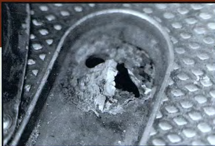
Results of a .50 Cal round that passed through the floor and exited through the greenhouse and the main rotors of Old Paint, "The Horse With No Name".
