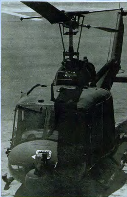
40mm turret on the nose & 14 2.75" rockets
