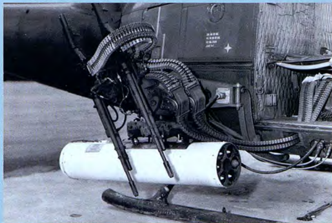
197th AHC Gunship equipped with quad 7.62 machine guns and two rocket pods (7, 2.75 inch rockets per pod)
