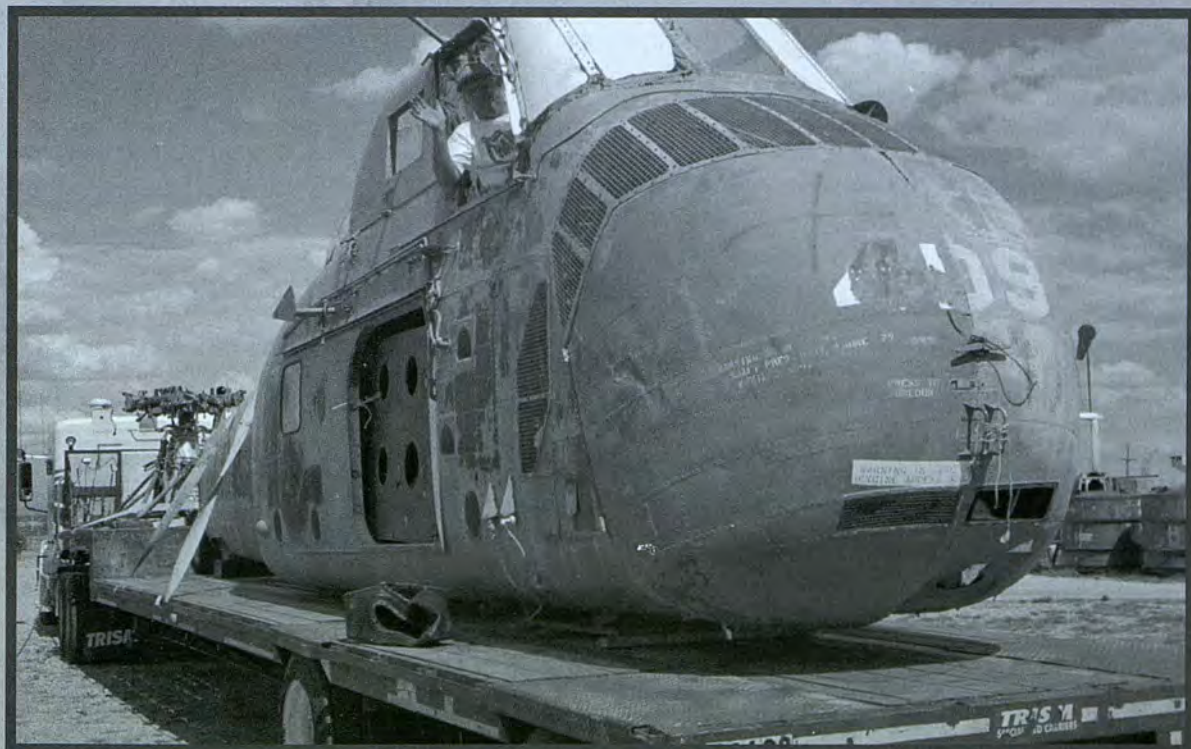
Aircraft on flatbed ready to go. Al Weiss is beaming in the cockpit. Note the transmission/rotor head assembly that is mounted in front of the airframe. The height of the UH-34D airframe necessitated removal to obtain adequate clearance under highway overpasses.
