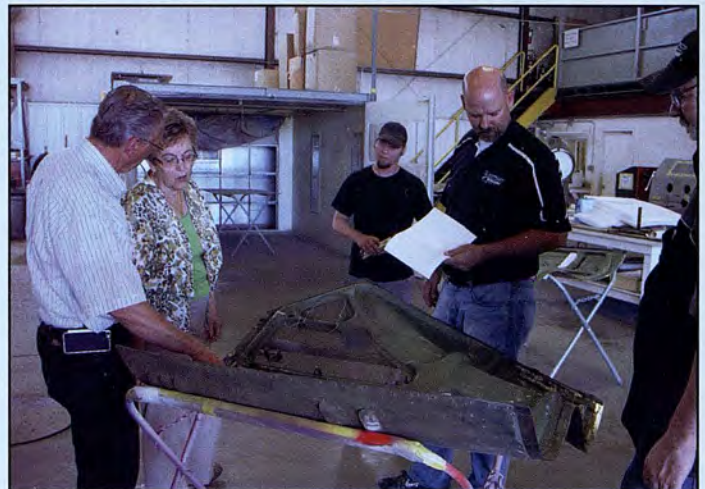
Larry and Karen Ayres discuss the details of the cowling with the Technician Team at Helicopter Specialties, Jon Fletcher, Jason Shrier, and Rick Theis. The cowling is a part of the turbine engine cover.
