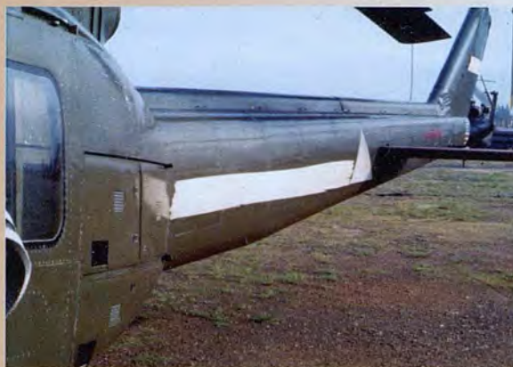
Taped over tail boom on the UH-1H.
