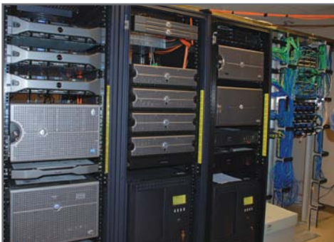
The Virtual Vietnam Archive started on one single-processor 70GB server in 2001, and now has expanded to a five box Server Area Network (SAN) with 32 processors and a storage capacity of 60TB.
